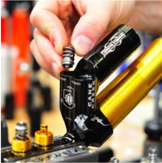
Install The poppet and spring
