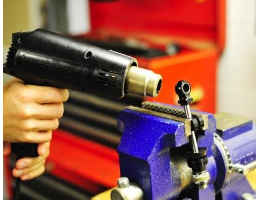
Use a heat gun to melt loctite before removal
