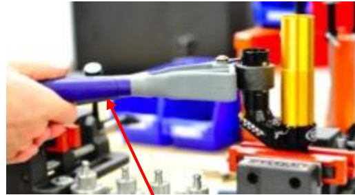
IFP Tool (measure depth before removal)
