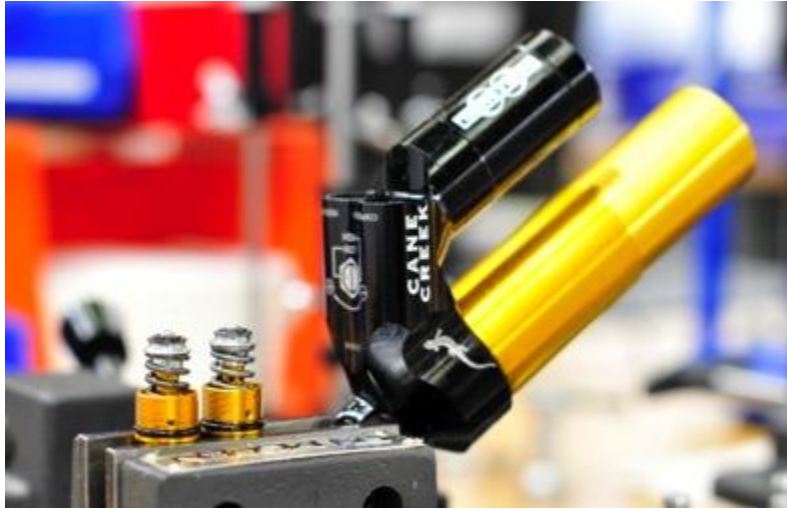
Poppet and springs removed from the shock head
