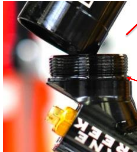
Lubricate o-ring
