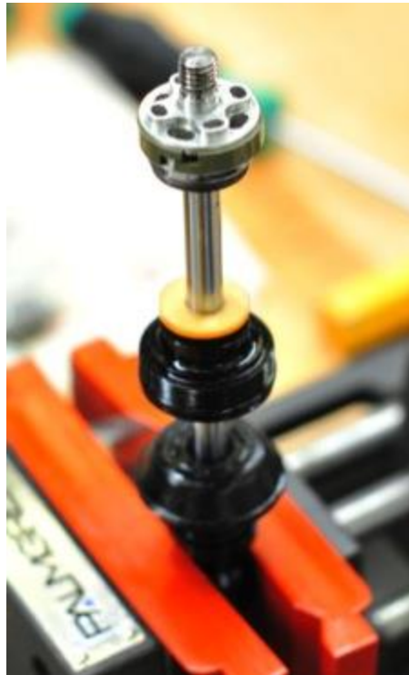
Correct orientation of the piston
