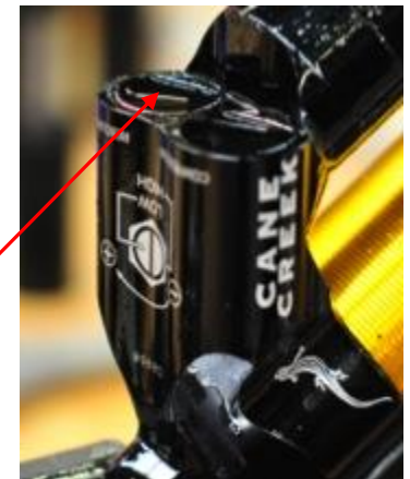
Fix the shock in a vice to start the fill process
