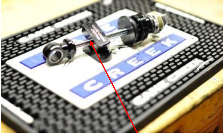
Secure damper shaft in a vice
