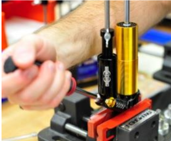
Screw the adjusters in to make circlip installation easier
