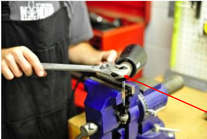
Secure damper shaft in a vice
