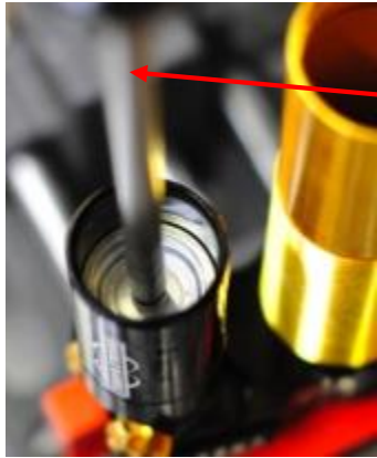
IFP Tool (measure depth before removal)
